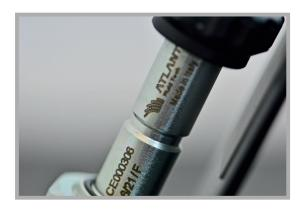
Special tubes have been designed to work reliably at the highest pressures. The employment of non-welded construction and the use of high-strength materials have produced valves that can work at 500 bar (7200 psi) with a burst pressure of 1300 bar (18800 psi).
