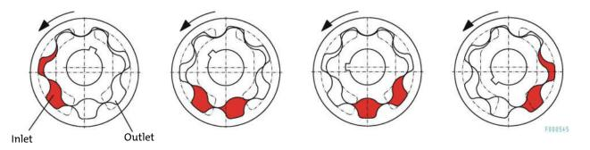
When we designed the BFP series we specifically selected the number of teeth and the width of the gerotors so the pumps have the smallest possible physical dimensions, low weight and minimal loss in efficiency. The low relative speed between the internal and external gear make the pumps extremely durable and smooth.
