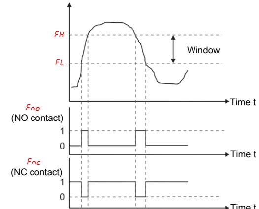
Example:  $F_{ILo} = 15^\circ\text{C}$ ,  $F_{IH} = 80^\circ\text{C}$
