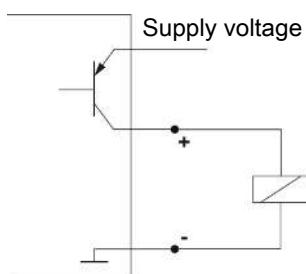
**Note:** When measuring the switching output with high-load measuring device inputs or when used as a frequency output, the load must be set to 10 kΩ between the output and earth (GND) to avoid faulty measurements.
