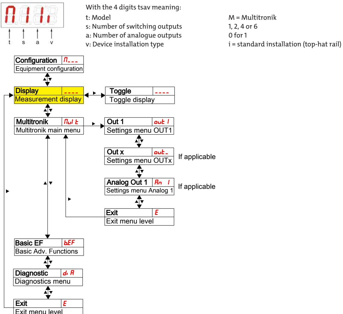
The individual menu items will not be shown if the option does not apply. Example: With a=0 the menu items for configuring the analogue output does not apply. You can then skip the description for this item.
