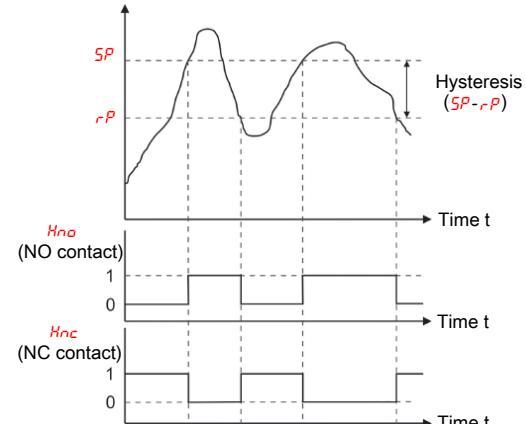
NO contact or NC contact function defining a signal window. When the measuring window is reached the output signal is set and deleted upon exiting.
