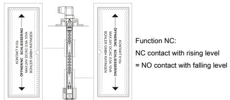
The contact logic assumes the level switch is installed in an empty tank, i.e. it is only in the operating position once filled.
