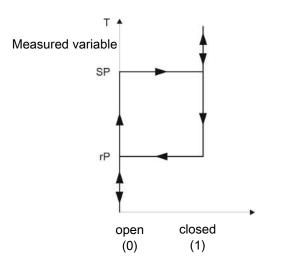
rising NO contact falling NC contact NO (normally open)
