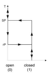
rising NC contact falling NO contact NC (normally closed)
