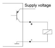
**Note:** When measuring the switching output with high-load measuring device inputs or when used as a frequency output, the load must be set to 10  $k\Omega$  between the output and earth (GND) to avoid faulty measurements.
