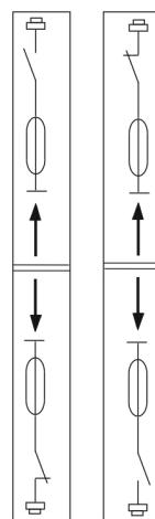
The contact logic assumes the level switch is installed in an empty tank, i.e. it is only in the operating position once filled.
