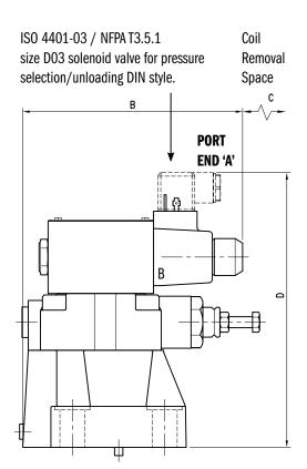
Hexagonal head main pressure adjustment screw: 13 mm [1/2] wrench Clockwise rotation to increase pressure.
