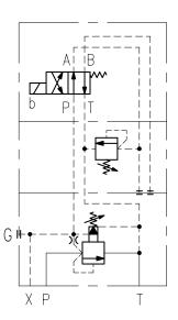
Pressure Relief, 2 pressure, normally low pressure, energize for high pressure
