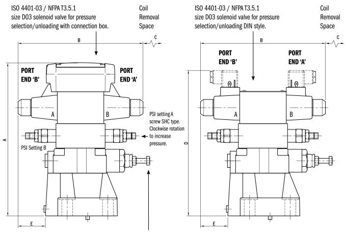
Hexagonal head high pressure adjustment screw: 13 mm [1/2] wrench Clockwise rotation to increase pressure.
