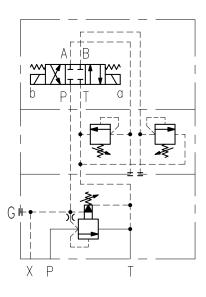
Pressure Relief, 3 pressure, normally highest pressure, energize A solenoid for pressure setting A energize B solenoid for pressure setting B
