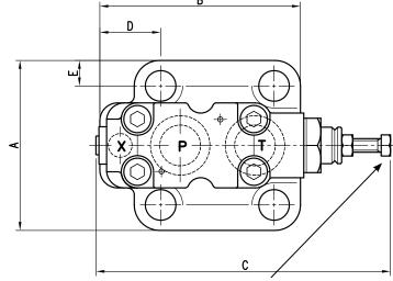
Hex cap adjustment screw (standard): 13 mm [1/2] wrench Clockwise rotation to increase pressure.
