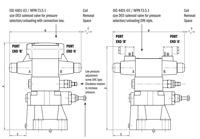
Hexagonal head high pressure adjustment screw: 13 mm [1/2] wrench Clockwise rotation to increase pressure.
