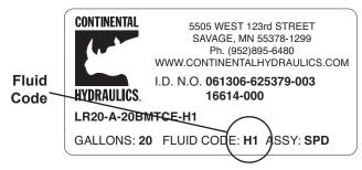
If the fluid you are using does not match the code on the label, contact your nearest Continental Hydraulics Representative before operating the power unit.
