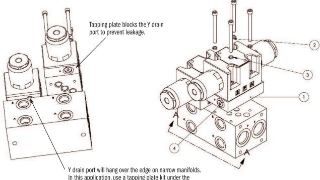
Y drain port will hang over the edge on narrow manifolds. In this application, use a tapping plate kit under the directional control valve to block the port. Use a manifold with a D05 alt A mounting pattern for applications where the drain port is required.
