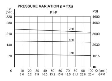
The curves have been obtained with inlet pressure 50 bar greater than nominal pressure.
