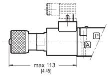
$\mbox{M}$  - Push and twist manual override (only for DC solenoid valve) Code:  $\mbox{M3401150026}$
