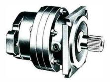
The CROSS Series 50 PGR gear reducer is a high torque, low speed unit with a peak output of 10,000 in. lbs. and a maximum continuous output torque of 8,000 in. lbs. This 5.33 to 1 planetary reducer also provides a radial load capacity almost double that of competitive units. Designed for use with the Cross 50 Series hydraulic motors, or other equivalent motors, they may be used for many general mechanical speed reduction or increase applications.
