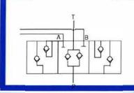
The CROSS series SS directional control valve offers extremely low leakage with exceptional load holding ability in a small, yet rugged, sectional valve. A single section may be utilized by itself or stacked in series to perform multiple functions giving this valve a unique versatility. Solenoid as well as manual actuators are available. It is compact, yet large enough to accommodate quick disconnect fittings.
