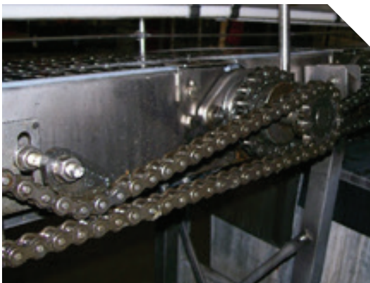
Multi-stage roller chain drives on a conveyor wore unevenly, creating synchronization problems.
