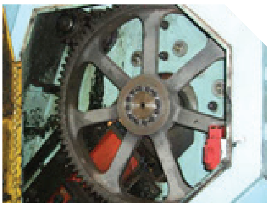
Bull gears on a stamping press needed replacing every three months due to wear.
