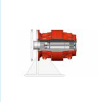
▲ Bracket mounted motor with flange adapter.
