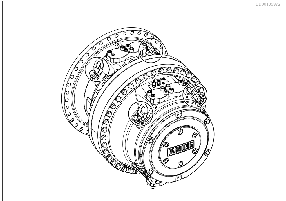
Fig. 4: Lifting eyes are included in delivery for CBp 280 to CBp 840
