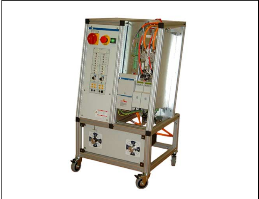
Abb. 5-1: 2-axis IndraDrive M demo system
