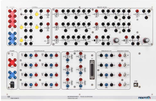
Figure 2: TS-EC-G-CR-SVAI operating unit (housing variant)
