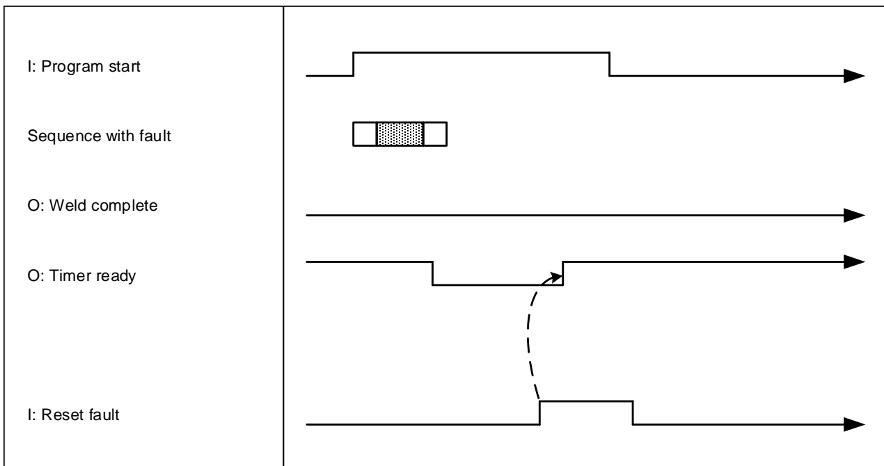
Fig. 10: Reset of a weld fault
