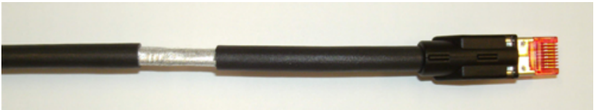
Fig. 10-18: CDI cable with partially removed jacket
