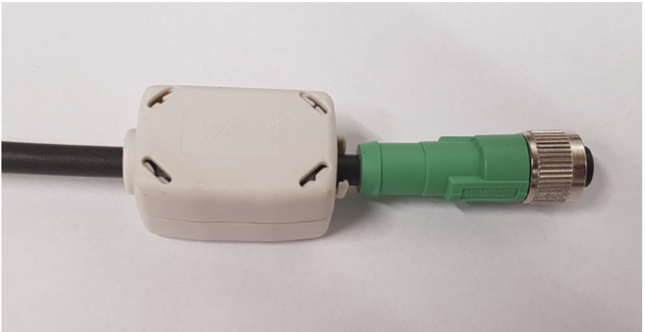
Fig. 9-3: Connection lead at X1S Power - Braid-breaker
