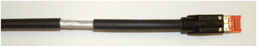
Fig. 10-13: CDI cable with partially removed jacket
