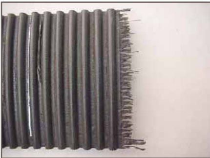
Figure 20 - Crimp failure due to debris
