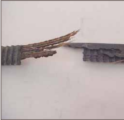
Figure 1 – Normal fatigue failure
