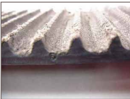
Figure 9 – Excessive tooth wear
