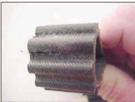
Figure 11 - Uneven belt wear
