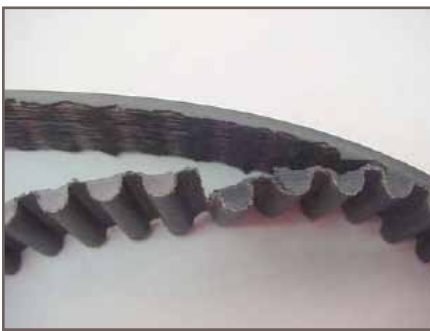
Figure 8 – Tooth separation failure
