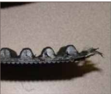
Figure 5 – Tooth root crack propagation
