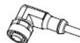
1024883 Female 90 DEG. Cord set; 5 m PUR-Cable M12 Connector; IP65; IP 67; IP 68; IP 69K Ambient Temp. -13-194 Deg. F (-25-90 Deg. C)
