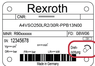
Fig. 5-2: Nameplate with direction of rotation arrow
