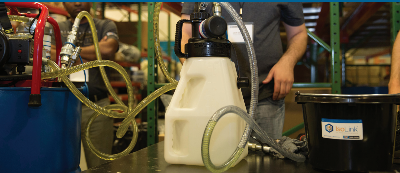
Figure 10: Small hand-held filtration with primary and secondary stage filtration suitable for contamination control within process pumps
