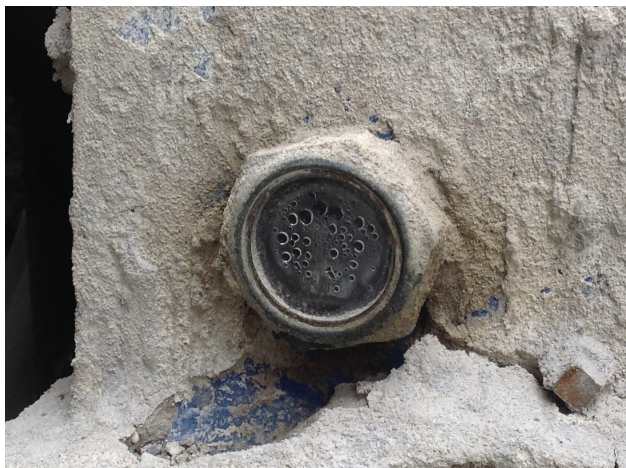
Figure 7: Replacing a flat sight glass with a 3D sight glass is a simple inexpensive modification that can greatly enhance the reliability of oil level checks.
