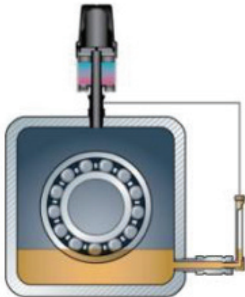
Figure 3: Optimum oil level for wet sump bearing lubrication for slow/moderate speeds is half way up the lowest rolling element
