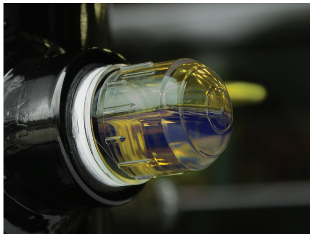
Figure 7: Replacing a flat sight glass with a 3D sight glass is a simple inexpensive modification that can greatly enhance the reliability of oil level checks.
