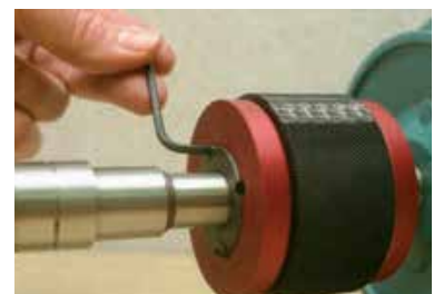
TIGHTEN SCREWS ALTERNATELY.
