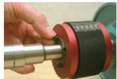
TIGHTEN SCREWS FINGER TIGHT.
