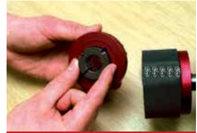
INSERT BUSH INTO END PIECE.
