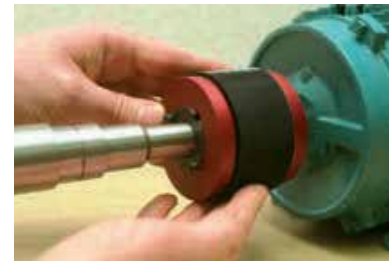
INSERT SCREWS AND LOCATE ON SHAFT.
