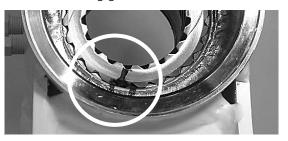
piston sleeve (3). Use a plastic mallet and mandrel if necessary. Avoid scratching or denting the inside of the housing bore.
