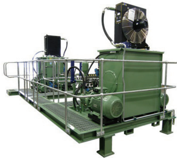
Return Line cooler on Hydraulic Power Unit.
