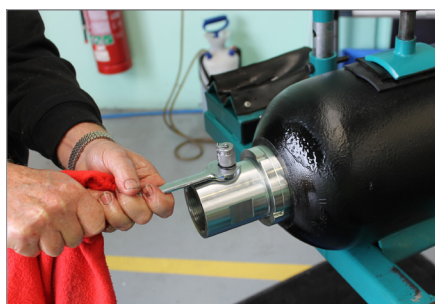
7. Remove the bleed valve on the fluid port.
