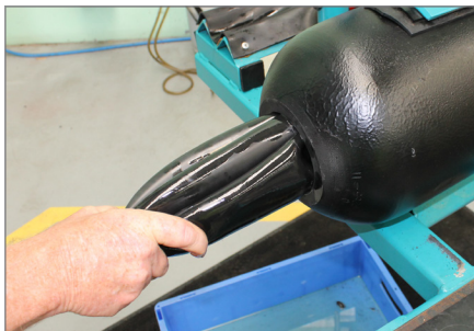
11. Remove as much air as possible from the bladder, then remove the bladder from the shell. DO NOT use any sharp objects that could damage the bladder.
