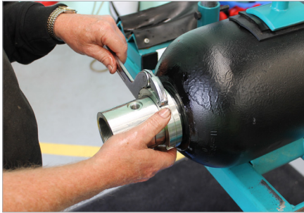
10. Remove flanged washer and locknut to enable installation of nylon back-up washer.
