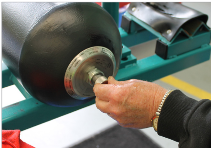
16. Fit the gas valve assembly cap.
