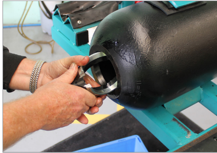
10b. From inside the shell slide the anti-extrusion ring off the fluid port body. Fold ring and remove from the shell.
