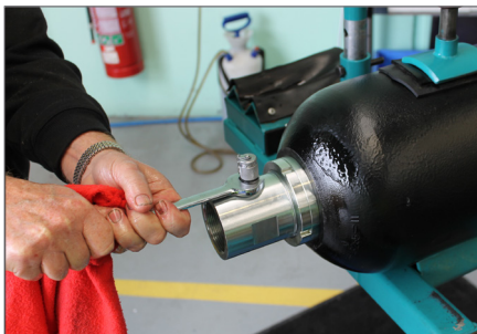
13. Fit the bleed plug or STAUFF test coupling (if fitted) and tighten.
