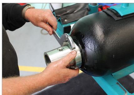
8. Remove the fluid port locknut with an appropriate "C" spanner along with the flanged washer.
