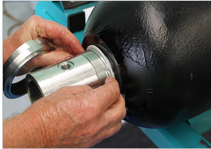
11. Ensuring the fluid port body does not get dislodged - insert the nylon back-up washer so that the concave face on the washer faces the O-Ring.
