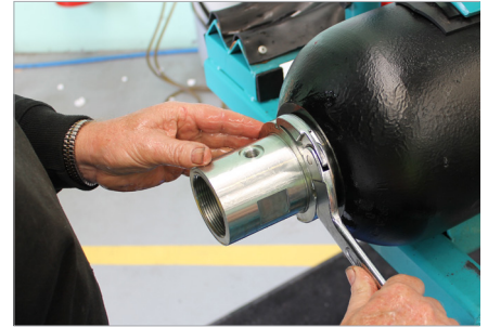
12. Attach first the flanged washer and then the locknut. Ensure the locknut is tightened using an appropriate spanner.
