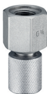
SDA-20-G1/4-W3 Adaptor for process connection G1/4 (B04) on test coupling STAUFF Test 20 (connection thread M16 x 2)
