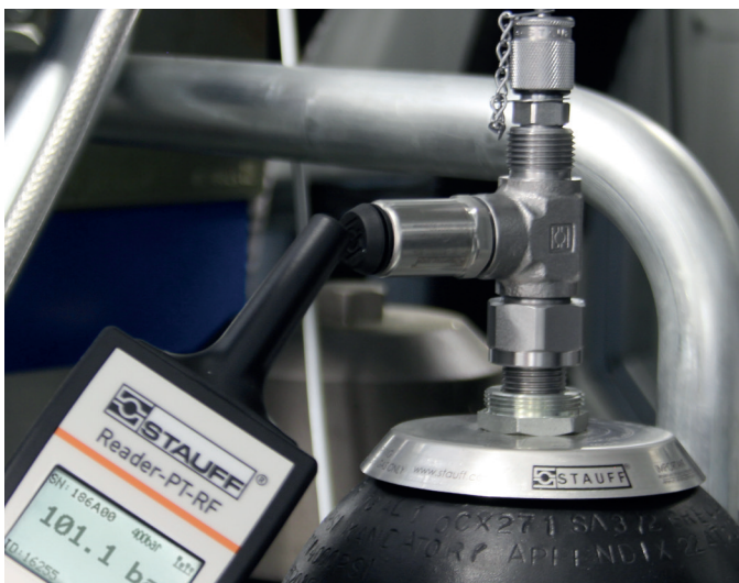
Bladder accumulator in use with Reader-PT-RF
