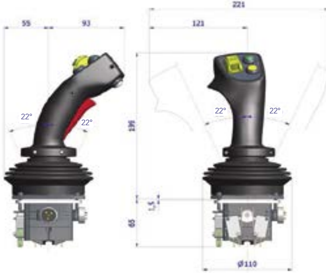
JMF base with MG type handle Complete code: JMF-L4C/NN-MG A2P9 1FPR R1P9
