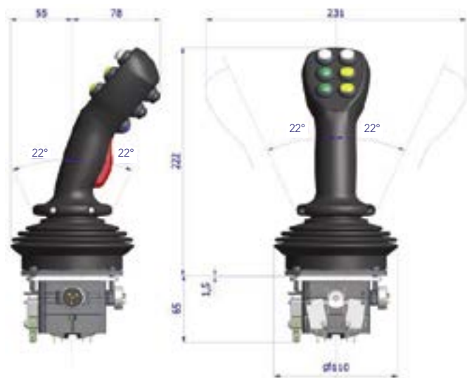
JMF base with MS type handle Complete code: JMF-L4C/NN-MS A6P9 R3P9
