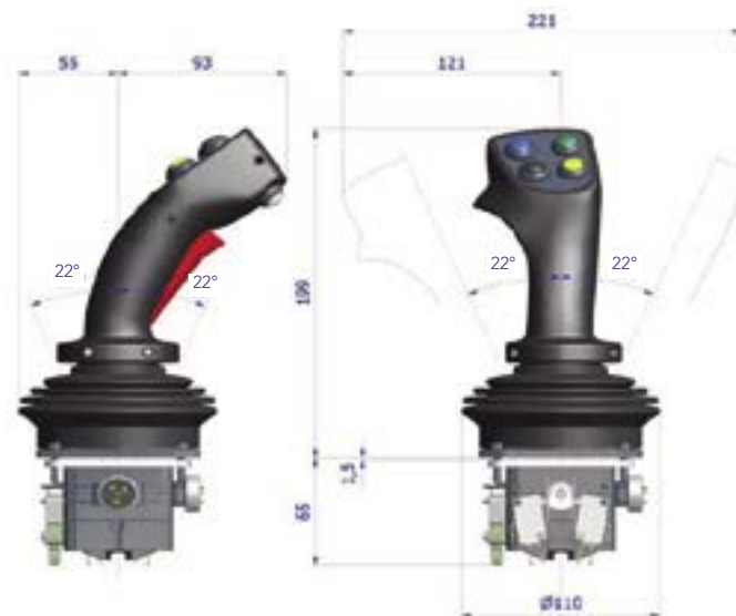
JMF base with MG type handle Complete code: JMF-L4C/NN-MG A4P9 R1P9
